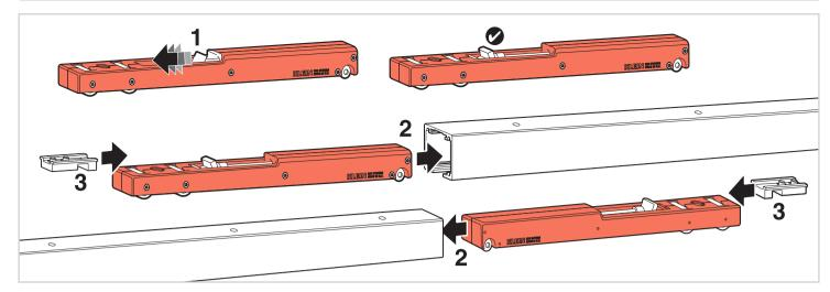
4 MONTAJE DEL PERFIL / UPPER TRACK MOUNTING
