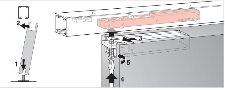
8 AJUSTE DEL PERNO / BOLT ADJUSTMENT
